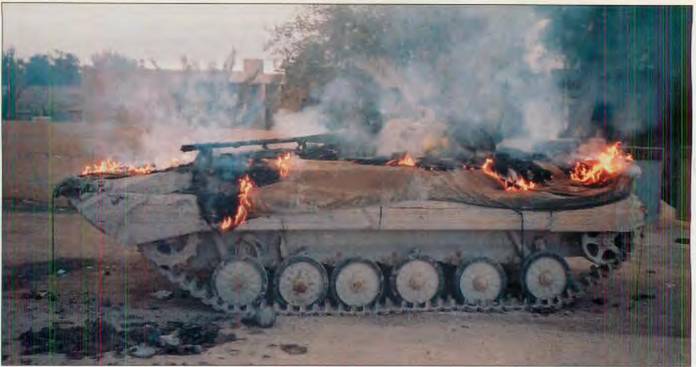
**Soviet designed IFV is toast after encounter with Marines' Mk-19 fully automatic 40 mm grenade launcher. Each 40 mm round can blow through 2.5 inches of steel easily burning multiple holes in this BMP-2.**
