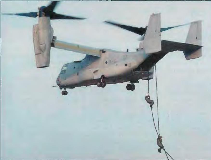
*(above) Design characteristics of V-22 make it a superior rotor-wing craft for such missions as HALO ops, but close to the ground for fast-roping (inset) it is vulnerable to ground fire, and its own problems with vortex ring state.*
