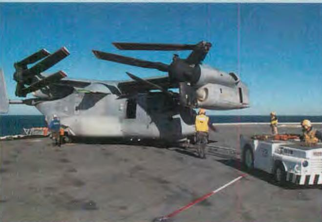
**On board suitable ships, hybrid Osprey re-oriens its fixed wing, folds its props/rotors for stowage.**
